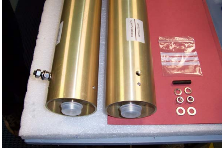
Figure 6: Photograph of Earthing Stud Connection for the W360
