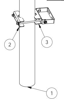
4. Using the above table, position the antenna in desired downtilt position. After positioning install the 5/16 locking hardware on both sides.
