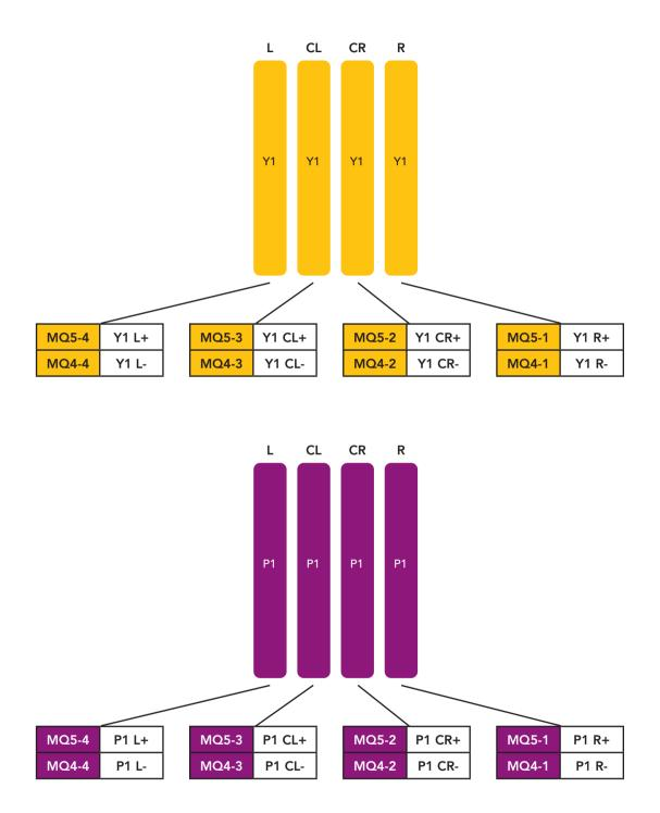
Physical array and port mapping according to AISG naming convention: Left - Center Left - Center Right - Right (seen from front of antenna)
