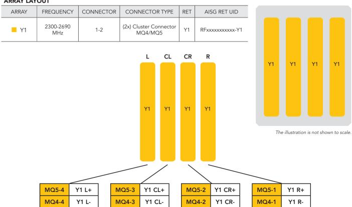
Physical array and port mapping according to AISG naming convention: Left - Center Left - Center Right - Right (seen from front of antenna)
