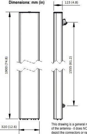
This drawing is a general representation of the antenna - it does NOT accurately depict the connectors or radome shape.
