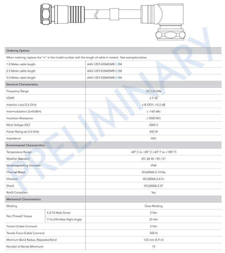
Quoted performance parameters are provided to offer typical, peak or range values only and may vary as a result of normal testing, manufacturing and operational conditions. Extreme operational conditions and/or stress on structural supports is beyond our control. Such conditions may result in damage to this product. Improvements to products may be made without notice.
