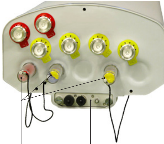
Location of the MDCU for RET Control
