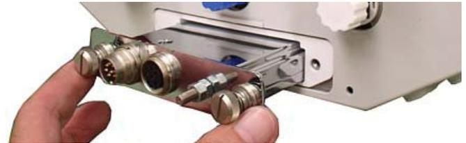
The module must enter freely. DO NOT force it. Rather, try to reverse the orientation. When the module is close to the end, increase pressure slightly to mate the internal connectors.
