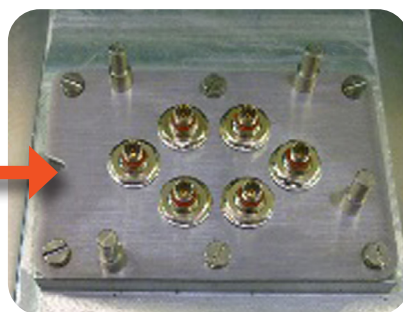
Blind-mate system on locomotive roof
